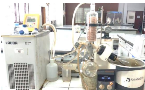
Vacuum rotary evatorator
