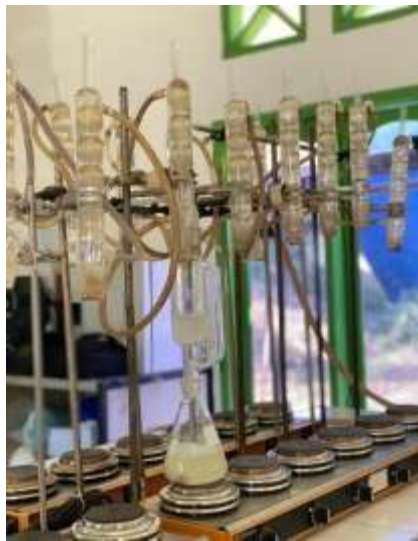
Gambar 8. Proses destilasi air nira aren
