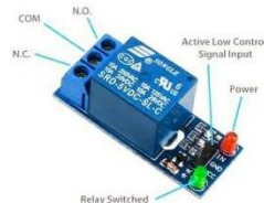
Sumber : E-Book MC Trainer ESP-32 MonsterChip Indonesia Gambar 2. 8. Module Relay Tanpa Optocoupler
