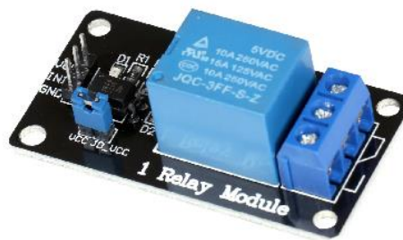
Sumber : E-Book MC Trainer ESP-32 MonsterChip Indonesia Gambar 2. 9. Module Relay Optocoupler
