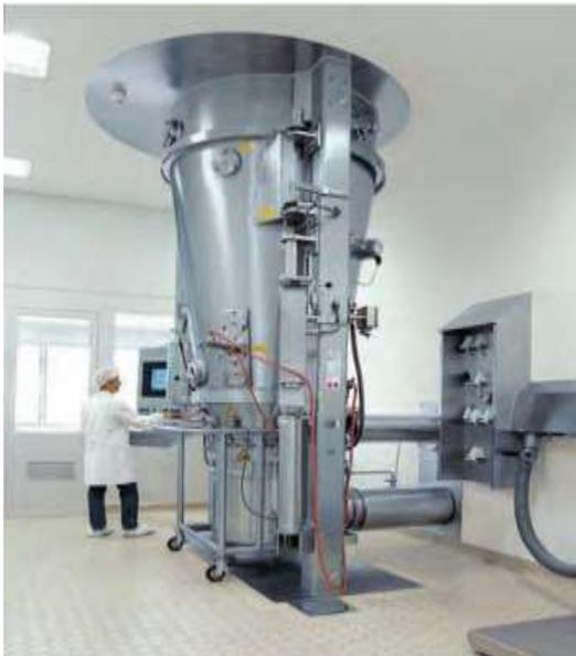
**Gambar 6.6.** *Fluidized bed granulator*
