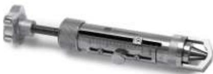
**Gambar 11.2.** Hardness tester
