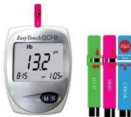
**Gambar 2.7** Alat hemoglobin metode *Point Of Care Test* (POCT).
