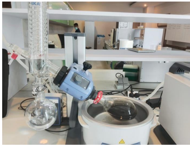
Rotary vacuum evaporator
